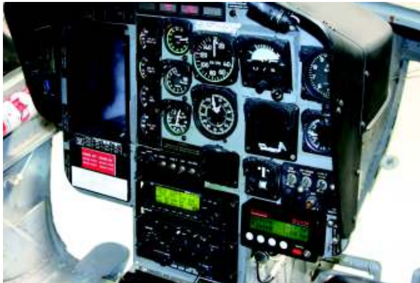
above: Perkins’ DAAM monitoring system installed in his Kiowa, at the bottom right of the cockpit.
